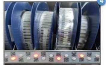
LED Indicator automatically combined display
